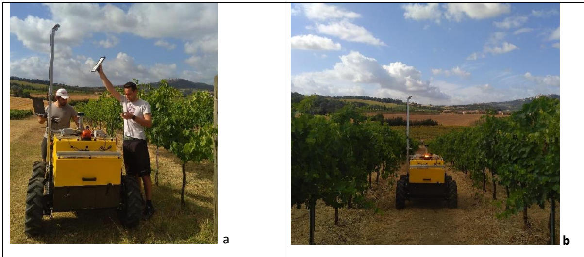
Figure 5. (a) & (b) An electric traction, self-driving prototype designed to move inside of vineyards through satellite systems advanced (GPS, RTK and IMU technology). It is equipped with a multispectral camera to capture the spectral signature for characterizing the vineyard health. The collected data is used to obtain vigor maps calculated using the NDVI index.
